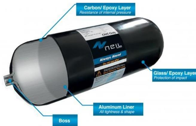
Figure 2. Composite Cylinder from NEIL [16]
